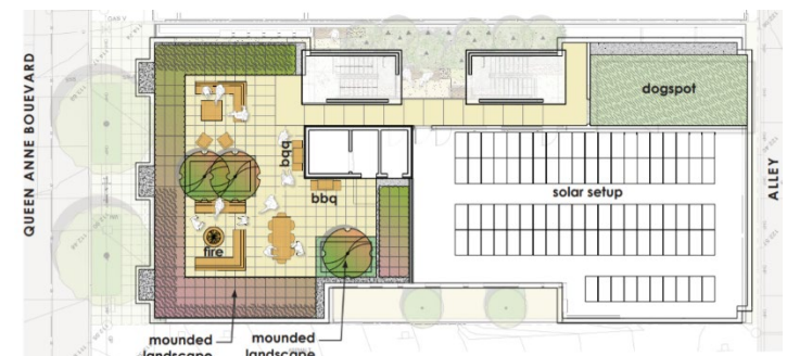
Roof Deck Plan with Solar PV array
